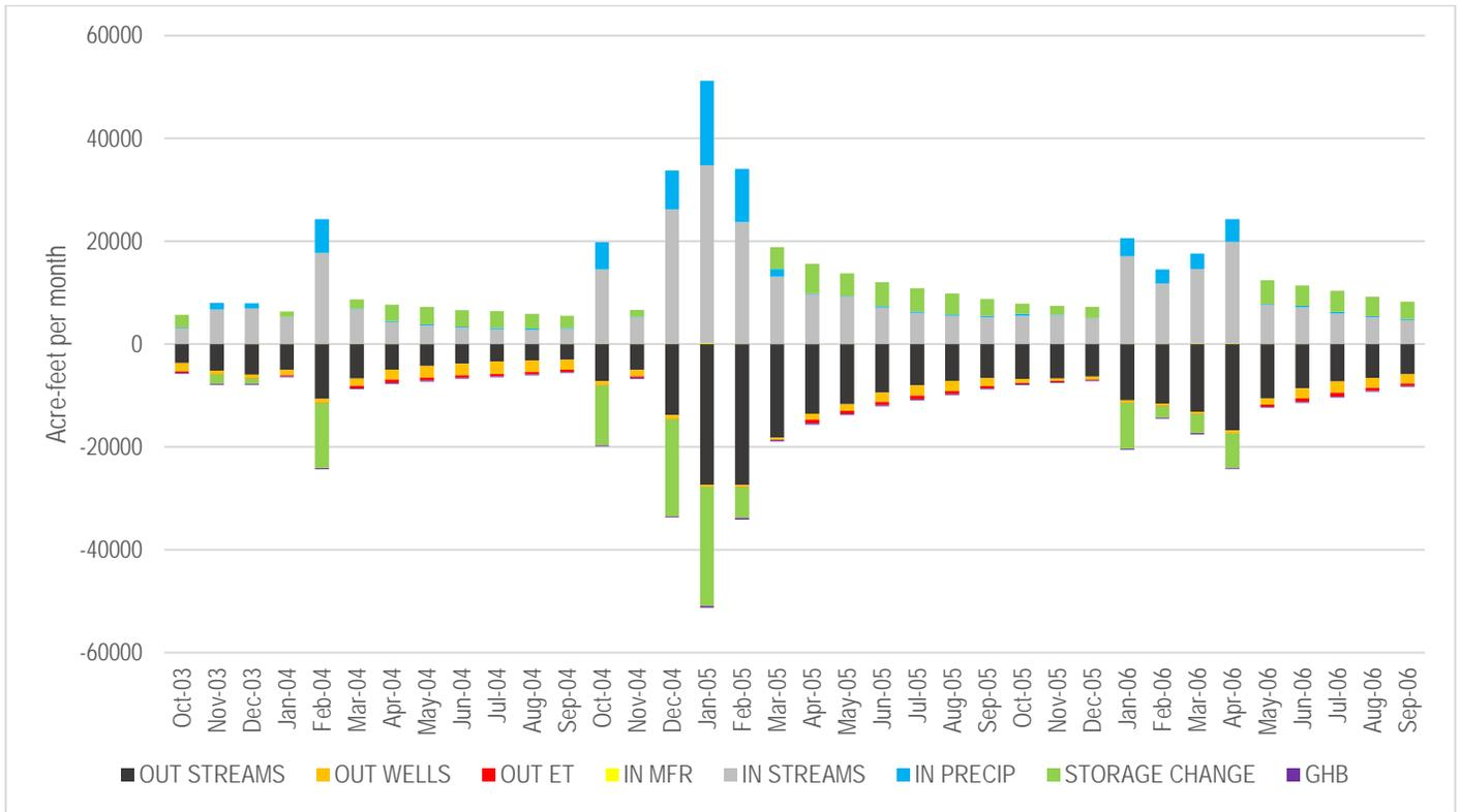
Figure 26. Simulated water budget over the 3 year calibration period. Negative storage change reflect a rising groundwater table; positive storage change indicates a lowering water table. ET= evapotranspiration; MFR= mountain front recharge; GHB= general head boundaries; OUT STREAMS= groundwater contribution to streamflow; IN STREAMS= surface flow contribution to groundwater
