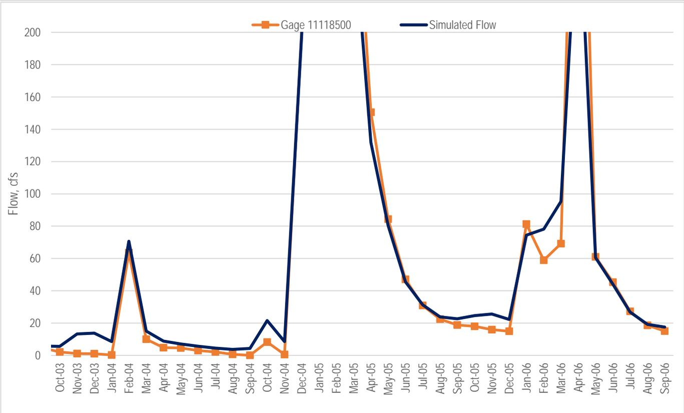
Figure 25a. and b. Average daily flows at USGS gage 11118500 (VCWPD 608) versus model simulated flow at the corresponding SFR segment for each stress period during the calibration period. A shows the full range of flow values, while B shows only flows up to 200 cfs.
