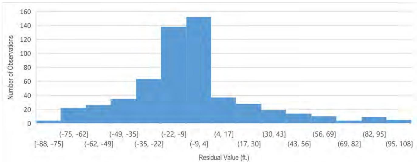
Figure 23. Histogram of all head residuals (observed-simulated) during the model calibration period. Each bar represents the number of observations with residuals in that bin. Residual values for each bin are given on the x-axis, where brackets indicate the upper bound (inclusive) and parentheses indicate the lower bound (exclusive).
