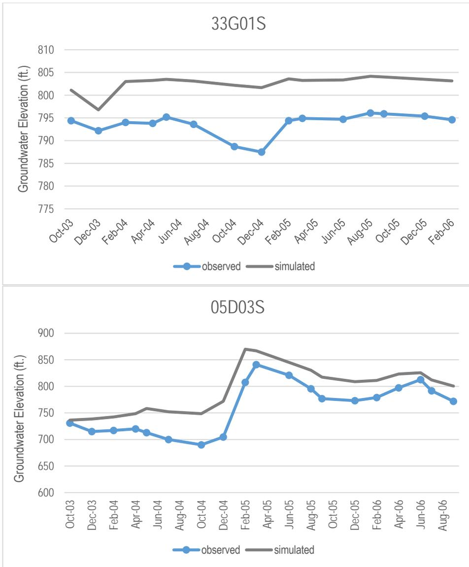
Figure 24b. Individual well hydrographs for observation wells in the Ojai Basin.
