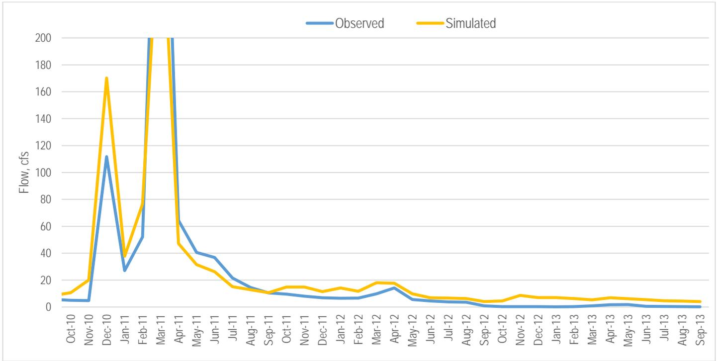
Figure 27. Observed (USGS Gage 11118500) versus simulated monthly streamflow during the model validation period.
