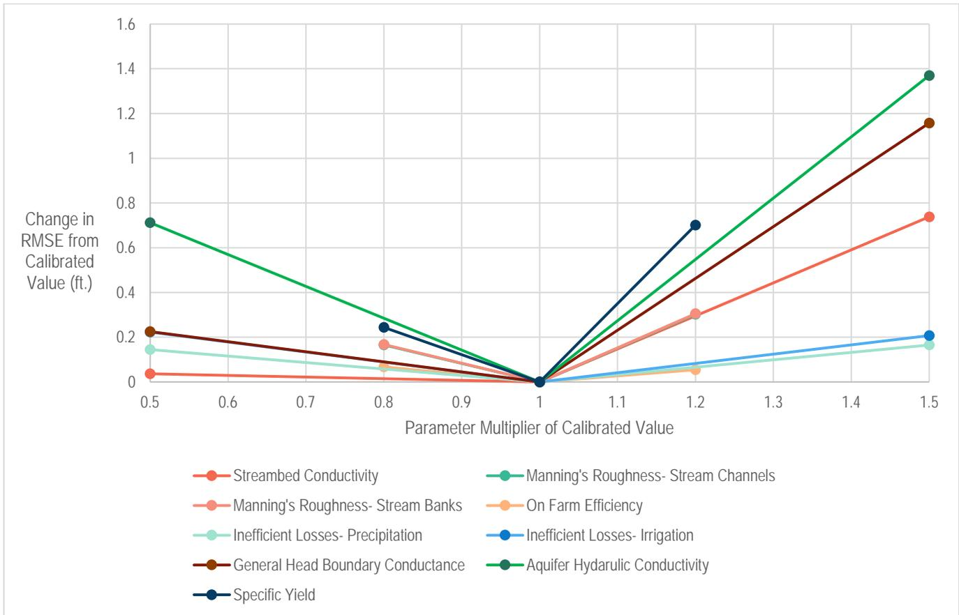
Figure 21. Results of the sensitivity analysis. Calibrated parameters are plotted as the parameter multiplier versus the absolute change in RMSE that resulted from altering the parameter.
