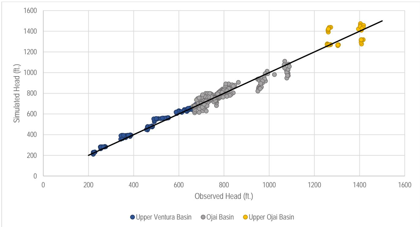
Figure 22. 1:1 plot of observed versus simulated heads during the model calibration period. The black line indicates a 1:1 relationship between heads.
