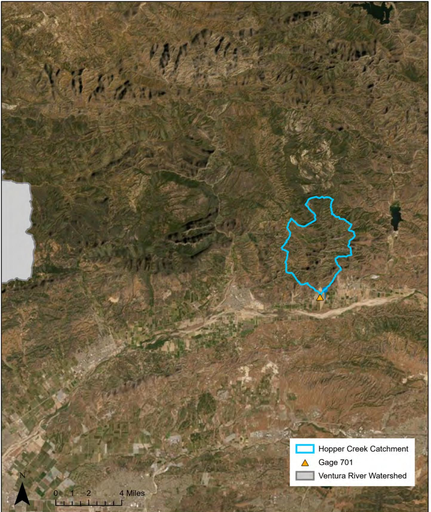
Figure 13. Precipitation Runoff Modeling System (PRMS) Calibration Catchment: VCWPD Gage 701, Hopper Creek at Highway 126 Santa Clara River Watershed
