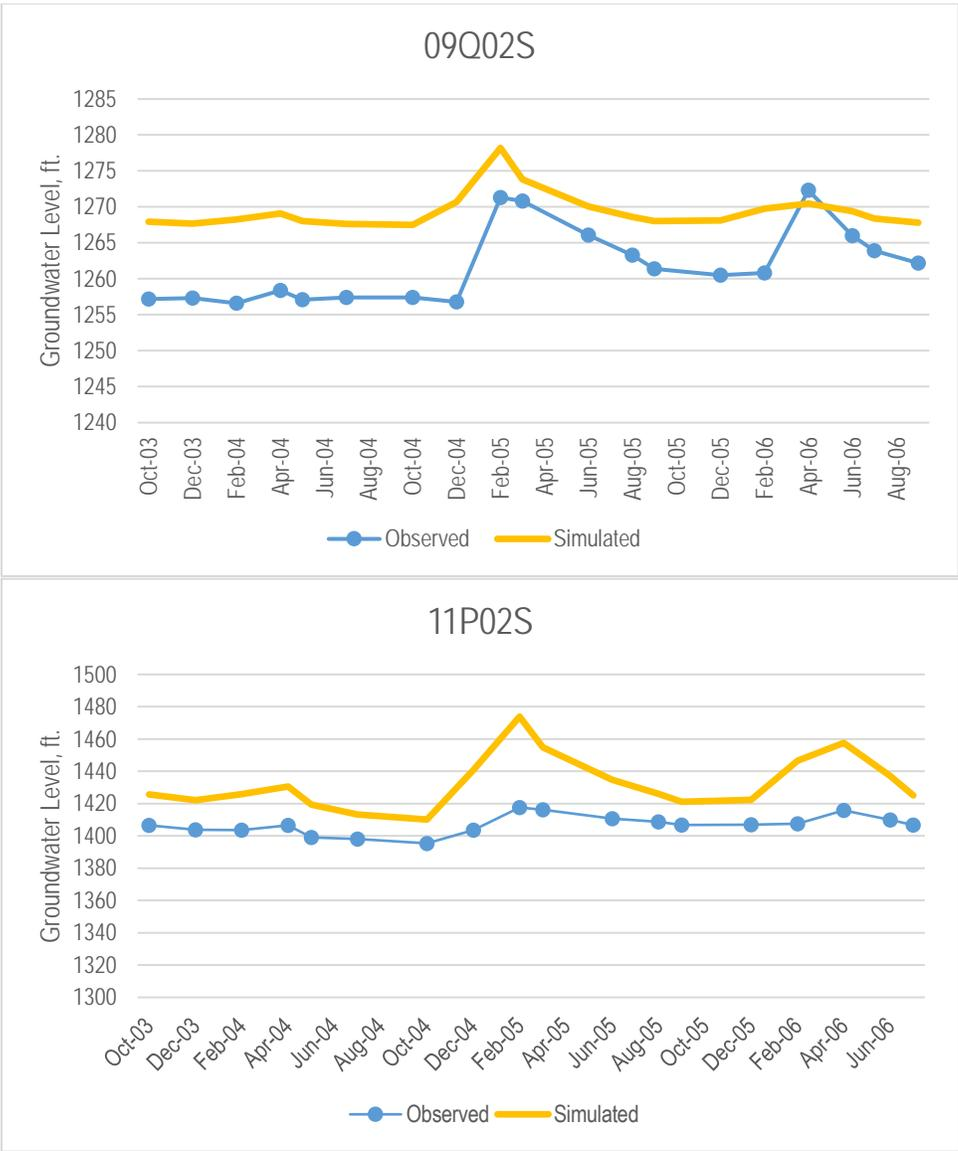
Figure 24a. Individual well hydrographs for observation wells in the Upper Ojai Basin.
