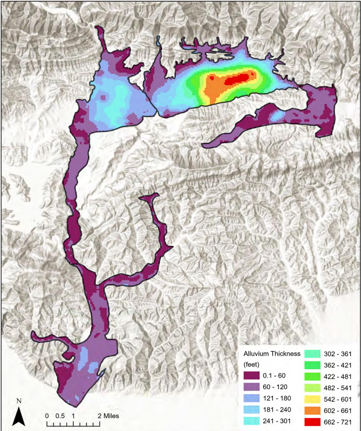
Figure 7. Model Alluvium Thickness
