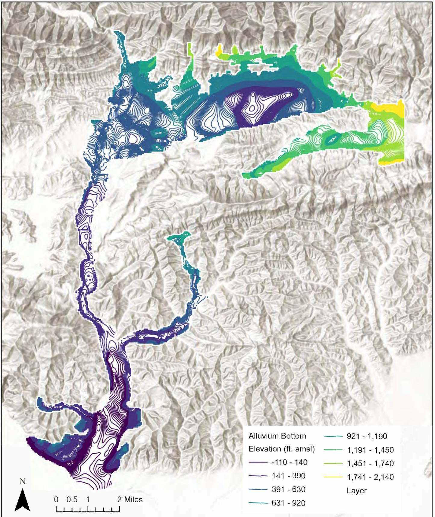
Figure 6. Layer 1 Alluvium Bottom Elevation Contours
