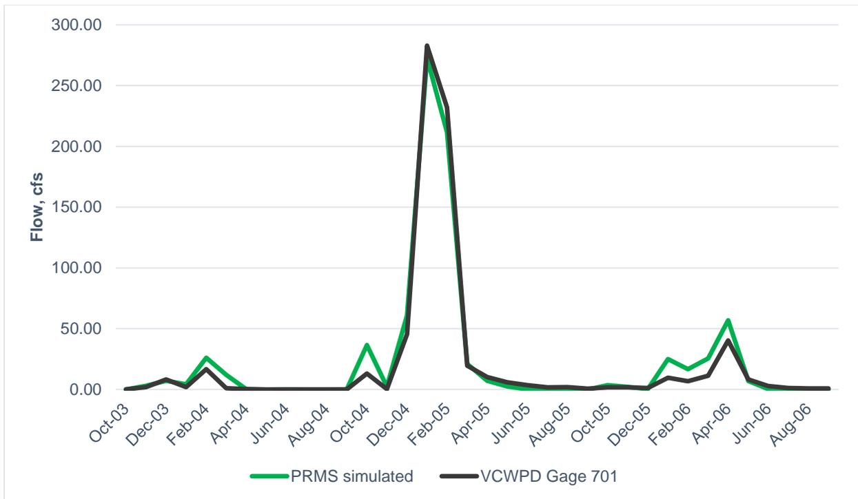
**Figure 14.** Plot of monthly average streamflow observed at the Ventura County Watershed Protection District (VCWPD) Gage 701, Hopper Creek at Highway 126 versus simulated streamflow by PRMS.
